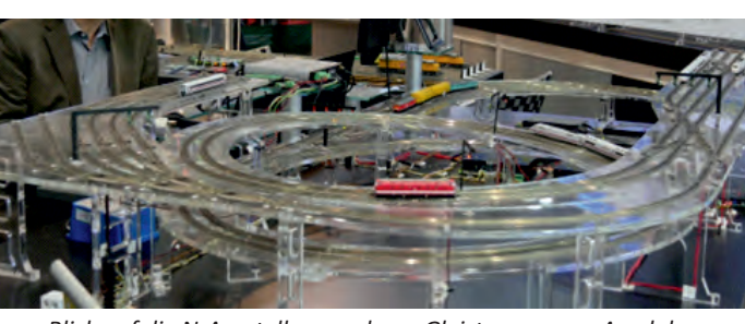
The ESTWGI interlocking for the ZIMO N-gauge layout: The purely technical demo layout is 2 x 1.3 m big, includes 3 stations with a total of 14 tracks, 3 routes with block operation and 1 reversing loop. The electronic equipment consists of an MX10 command station with (usually) at least 2 cabs (currently MX33), and 8 StEin modules; there are special ones for the signal bridges, some with integrated accessory decoders MX820, partly with modified StEin signal boards.
